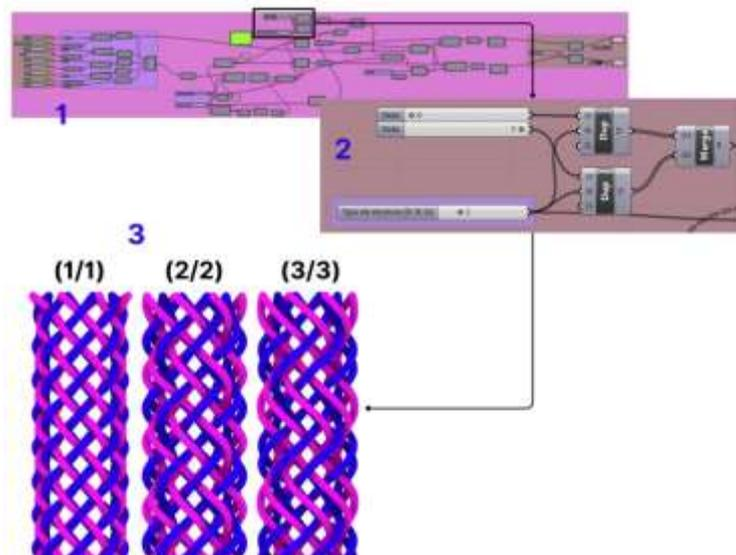
Figure 7. 1. In pink, the complete structure of the algorithm. 2. Part of the algorithm responsible for defining the parameter/type of structure regarding the ligament. 3. The types of structures resulting from the definition of the ligament, Diamond (1/1); Regular (2/2) and Hercules (3/3).
