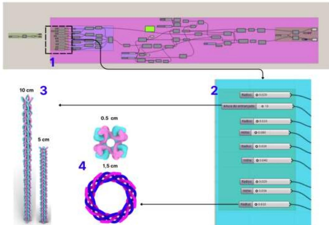
Figure 10. 1. In pink color, the complete structure of the algorithm. 2. Part of the structure responsible for “extrusion” and regulation of the yarn diameter. 3. The types of yarns with different dimensions, respectively 0.30mm and 0.60mm.
