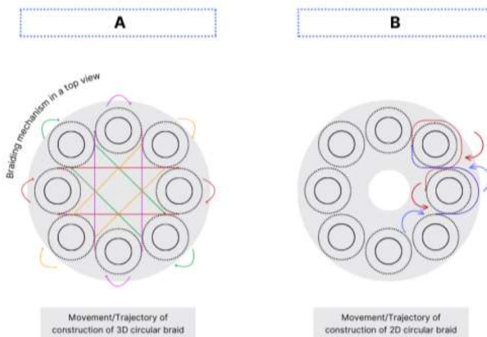
Figure 1. Machine movement/trajectory for the construction of interlaced geometries. **Group - A:** 3D circular hexagonal interlacing. **Group - B:** 2D circular interlacing.
