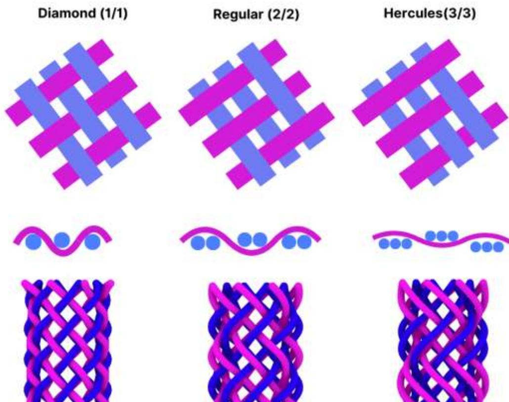
Figure 3. Braided structures with a model representing the ligaments. The three most common types of braided structures—Diamond (1/1), Regular (2/2), and Hercules (3/3)—are also illustrated. These structures were designed using algorithmic programming with Rhinoceros 3D® software and Grasshopper plugins.
