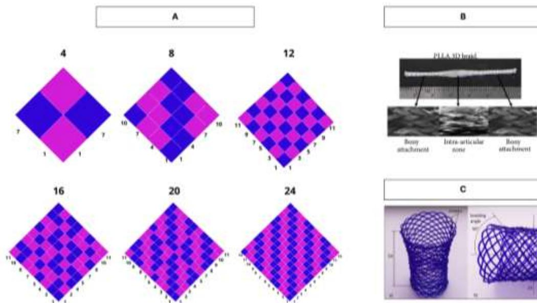
Figure 2. Group - A: Braided structures using varying numbers of yarns on a 12-gear Horngear braiding machine. Group - B: Braided scaffold structure for ACL ligament repair (Source: adapted from James & Laurencin, 2014). Group - C: Stent-type braided structure (Source: adapted from Shanahan et al., 2017).
