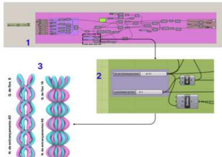
Figure 8. 1. The complete structure of the algorithm is shown in pink. 2. A section of the structure responsible for defining the number of braids and the number of strands. 3. The types of structures resulting from modifications in the parameters for the number of strands and number of braids.
