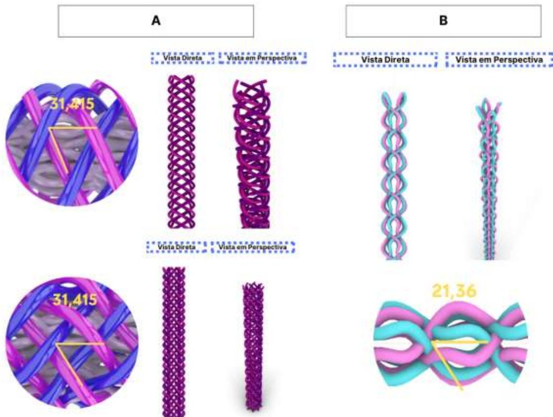
Figure 11. **A.** Graphical representation of the textile structure of the outer layer, produced using the software. Structures with 8 yarns and 16 yarns, with an average angle of  $\pm 31.415^\circ$ . **B.** Graphical representation of the textile structure of the outer layer, produced using the software. Structure with 8 yarns and an average angle of  $\pm 21.36^\circ$ .
