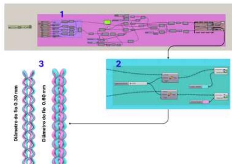
Figure 9. 1. In pink color, the complete structure of the algorithm. 2. Part of the structure responsible for "extrusion" and regulation of the yarns diameter. 3. The types of yarns with different dimensions, respectively 0.30mm and 0.60mm.
