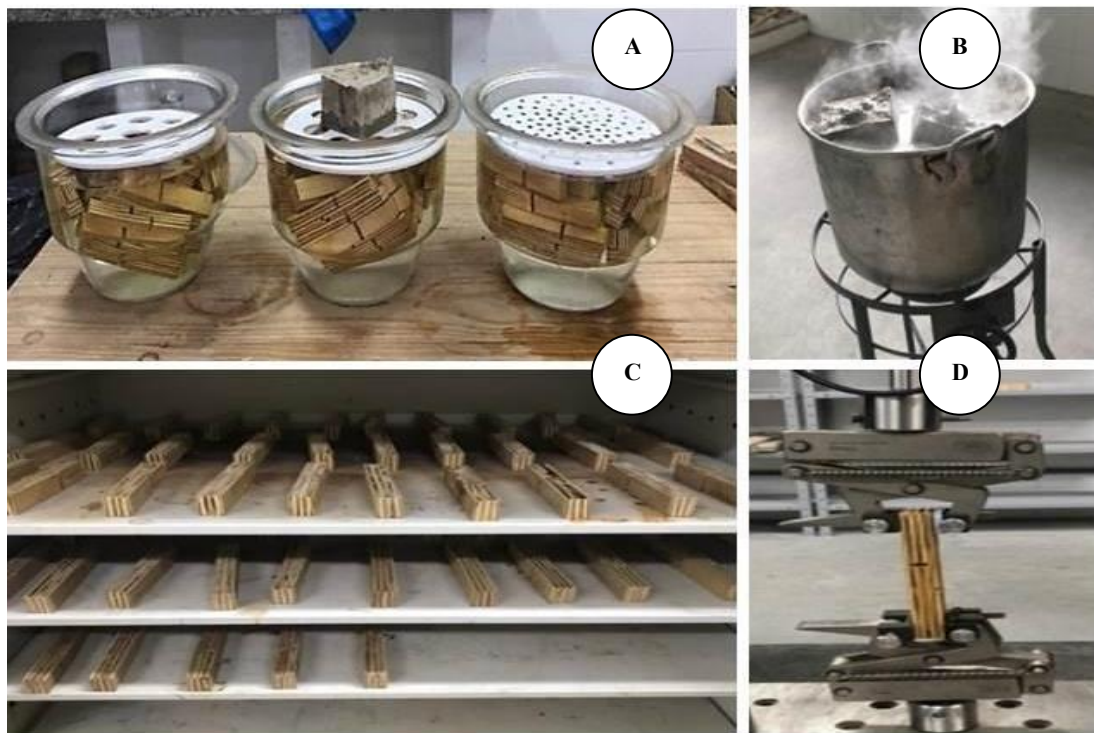
Figure 1. Steps for carrying out pre-treatments on the specimens before the shear strength test at the glue line. Specimens immersed in cold water (A), Specimens immersed in boiling water (B), Drying of specimens in a drying oven (C); Specimens subjected to the shear test at the glue line on a universal mechanical testing machine (D).
